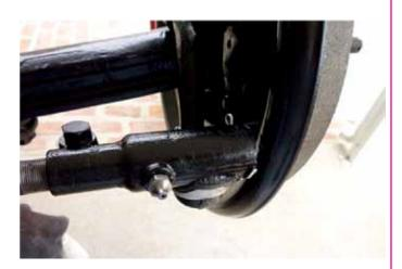
The right side (with the single spindle ball) has a left hand thread in both the tie rod and the tie rod end assembly. When installed, the grease fitting will face aft.
