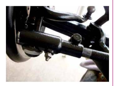
The left side (with the double ball spindle) has a right hand thread in both the tie rod and the tie rod end assembly. When installed the grease fitting will face aft.
