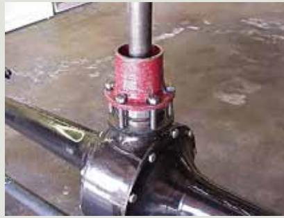
#18. The pinion gear assembly with the Mitchell stub shaft installed is re-inserted into the banjo using a tool made from a cut off torque tube. Tighten the six nuts evenly while rotating the stub shaft to engage the pinion gear with the ring gear. Continue tightening until the pinion assembly is fully seated.
