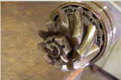
#14. Close up view. The cotter pin is to be removed and the nut backed off about 1/8". (Note that one leg of the cotter pin is bent over the end of the drive shaft. This should never be done as it may interfere with the rotation of the ring gear carrier. The correct method is to bend both legs of the cotter pin down along the side of the nut.)
