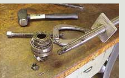
#16. The pinion assembly has been removed from the drive shaft with the existing pre-load still intact.
