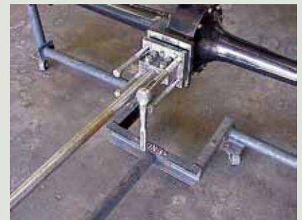
#7. A socket wrench is used to operate the drive shaft puller tool. Tighten each of the four bolts evenly.
