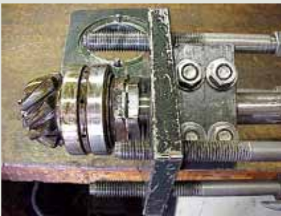
#11. Close up view before puller tool is removed. The four nuts and bolts holding the clamping device to the drive shaft are to be loosened and the device slid off the drive shaft.
