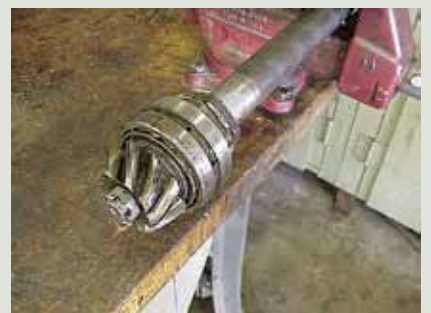
#13. The pinion gear and bearing assembly is ready to be removed from the drive shaft.
