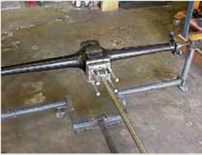
#5. The drive shaft puller tool is installed. It will pull the drive shaft and pinion assembly out of the banjo with the pre-load intact and not disturbed as long as the two large nuts are not loosened.
