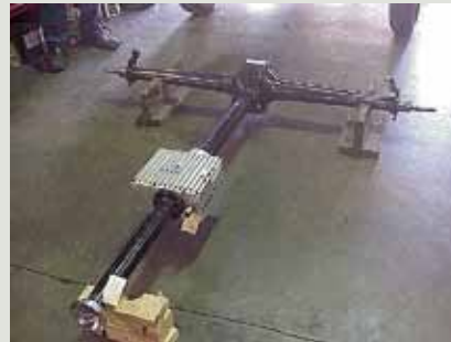
#21. The Mitchell overdrive installation is complete and the rear axle assembly is ready to be installed back in the car.
