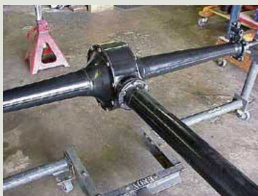
#2. Close up view. The torque tube is to be removed by removing the safety wire and the six mounting bolts. Remove the speedometer drive assembly and the snap ring in front of the speedometer drive gear before pulling the torque tube off. The torque tube, drive shaft, and the speedometer drive gear assembly will be discarded. Speedometer operation will be obtained at the output gear of the overdrive. An extension speedometer cable is supplied with the Mitchell overdrive that will connect to the existing speedometer cable.
