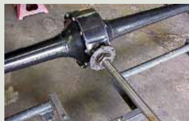
#4. Close up view. The drive shaft and pinion gear assembly is to be removed without destroying the pre-load on the pinion bearings. The use of a drive shaft puller is required. Do not loosen the two large nuts as it will destroy the pre-load.
