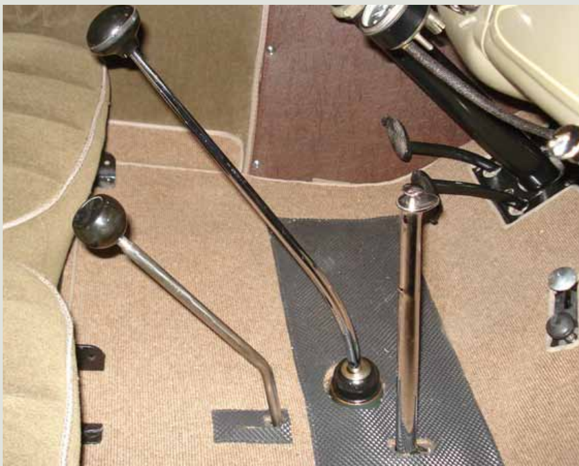
#23. The Mitchell shifter is located behind and to the right of the standard shifter. Shift it forward and you are in overdrive. Shift it aft and you are out of overdrive. The overdrive can be used in any gear and is particularly beneficial in second gear-overdrive when driving in mountainous terrain.
