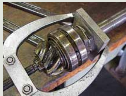
#15. A flywheel puller and a backing device are used to remove the pinion assembly from the drive shaft. Tighten the puller sufficiently tight and tap the end of the puller with a hammer. Continue tightening and tapping until the pinion breaks loose from the taper on the drive shaft.
