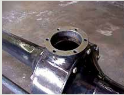
#9. Close up view of the banjo with pinion removed. Oil in the banjo does not have to be drained.
