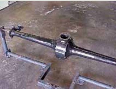
#8. The drive shaft and pinion gear assembly have been removed from the banjo. If the rear radius rods were still installed they can be supported in the front with a jack stand to keep the banjo flange horizontal to prevent oil from spilling out.
