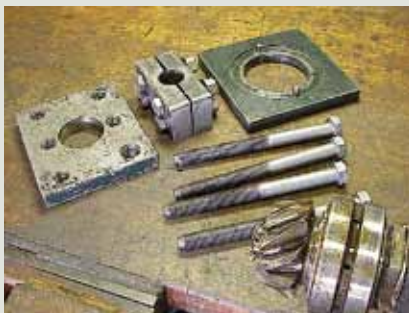
#12. Close up view of the individual parts of the drive shaft puller tool.
