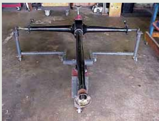
#1. The rear axle assembly is removed from the car and readied for the Mitchell install. It is not necessary to remove rear wheels, brake drums, backing plates, and rear radius rods.
