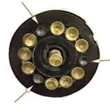
The second problem are the three Black OFF detents. They are .017 deeper resulting to make it harder to move out of the detent. Take a knife and scrap the edge of the hole to tapper edge.
